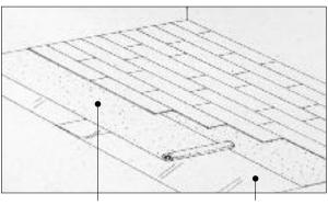
Pergo SilentStep<sup>™</sup> Foam or Soundbloc<sup>™</sup> Foam to be used with flooring that doesn't have attached underlayment. Vapor barrier over concrete – Moisturbloc™
