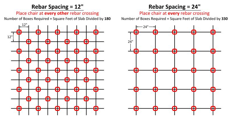
If rebar spacing is greater than 12", place chair at **every** rebar crossing. If rebar spacing is 12" or less, place chair at **every other** rebar crossing.
