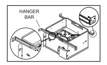
2b. Extend the hanger bars to the width of the framing. Position the ventilator with the hanger bar tabs wrapped around the bottom edge of the framing, holding the ventilator in place. Secure hanger bars to framing using one screw on each end of hanger bar. Select a proper hole and secure the hanger bars together using flange screws.
