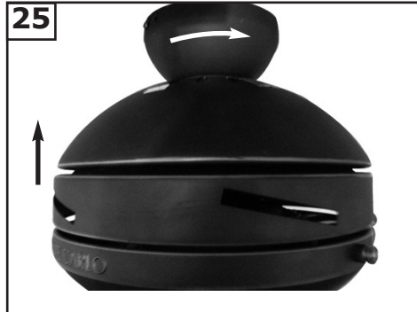
25 Lift fan to mounting bracket, aligning the "L" shape holes with the screws on the mounting bracket. Turn the fan clockwise to lock in position. Install the other 2 screws included in hardware bag and tighten all 4 securely.
