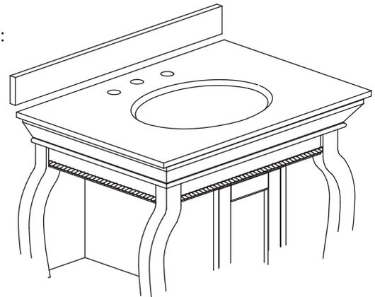
Finally, place the bottom side of back splash with sealant onto the countertop and check alignment of backsplash. Adjust the leg levelers as needed
