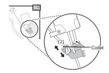
2 Remove the screw (1) from the hinge cover at the top of the refrigerator. Lift the hook (not visible), located at the bottom of the front side of the cover (2) with a flat-head screwdriver.
