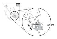
6 Place the cover (1) in place. Insert and tighten the cover screw (2).
