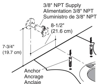
**6** Position brackets as shown on the template and install.
