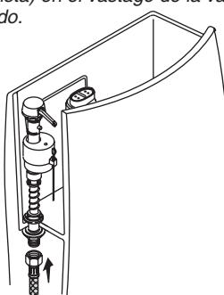
**8** Slide nut onto the supply hose, with flared end last and run hose through toilet wall.
