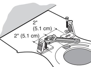
**7** Thread the supply hose (not supplied) onto the fill valve shank.
