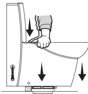
**13** Carefully thread the screws into the brackets, until toilet is secure. Alternately tighten left and right sides to prevent pulling the toilet off center. Install cap to cover screw.
