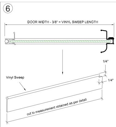
Measure Door width as shown and trim Vinyl Sweep to 3/8" less then measurement obtained. Notch one end of Vinyl Sweep one quater inch (approximate) as shown.
