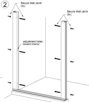
Position Jambs on sill, mark and drill 3/16" installation holes on walls. Insert Screw Anchors into holes and secure Wall Jambs to walls with 1-1/2" Installation Screws Provided. Note that adjustment holes are toward interior.
