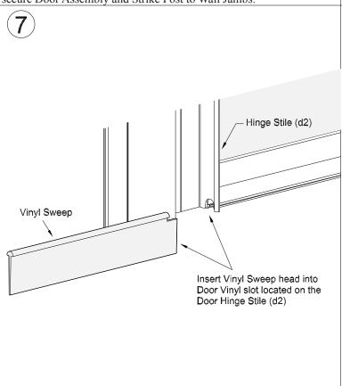
Insert Vinyl Sweep into Door Vinyl Slot as shown. Slot is located on hinge side of the Door Assembly.
