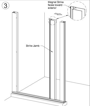
Decide which side you want your Door to strike and slide Strike Jamb into appropriate Wall Jamb (detail above shows unit will strike on right side).
