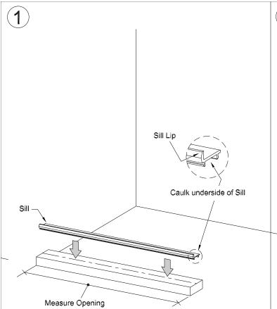
Measure opening width and trim sill to 1/16" less than measurement obtained. Caulk underside of sill and position it on center of curb. Insure that sill lip faces toward outside of enclosure.
