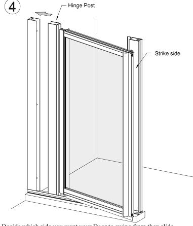
Decide which side you want your Door to swing from then slide Hinge Post into appropriate Wall Jamb (detail above shows unit striking on right side).
