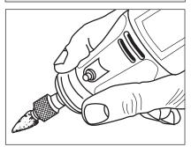
The first step in learning to use the Rotary Tool is to get the "feel" of it. Hold it in your hand and feel its weight and balance. Feel the taper of the housing. This taper permits the Rotary Tool to be grasped much like a pen or pencil. The #470 Variable Speed tool has a unique comfort grip on the nose and back seating, which allows the user added comfort and control during use. You can feel the difference!
