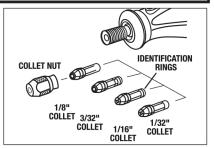
**COLLET NUT** - To loosen, first press shaft lock button and rotate the shaft by hand until the lock engages the shaft preventing further rotation.
