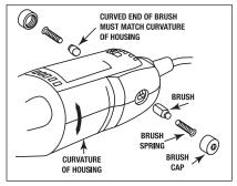
With the cord unplugged, remove the brush caps one at a time with a small screwdriver by rotating cap counter-clockwise and check each brush.
