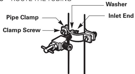
Route the tubing between the cold water line and the refrigerator.
