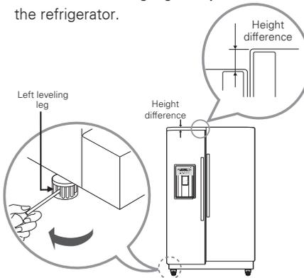
**NOTE:** Having someone push backward against the top of the refrigerator takes some weight off of the leveling legs. This makes it easier to adjust the legs.
