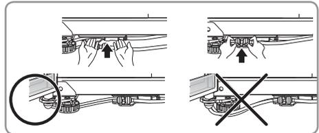
1. Feed the water tubes through the lower hinge pin and place the door onto the lower hinge pin. Water hoses should be behind the leg to prevent damage.
