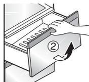
**NOTE:** When removing or installing the lower Fresh Zone drawer, lift the cover to help remove or insert the drawer.
