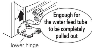
6. Place the door, inside facing up, on a non-scratching surface. Be careful not to damage the water feed tube.
