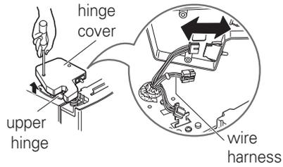
1. Open the door. Remove the top hinge cover screw.
