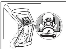
Rotate the water filter up into position and close the cover. The cover will click when closed correctly.
