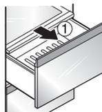
To install, slightly tilt up the front, insert the drawer into the frame and push it back into place.
