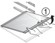
Remove all items from the shelf. Lift the front of the shelf slightly to disengage the rail stops.
