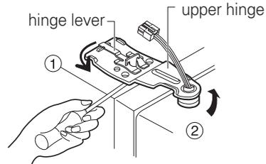
4. Rotate the hinge lever counterclockwise (1). Lift the upper hinge free of the hinge lever latch (2).
