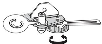
insert, open the freezer door and lift it at the lower hinge. Use a pliers to insert the ring on the lower hinge pin.
