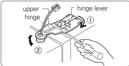
3. Rotate the hinge lever clockwise (1). Lift the upper hinge free of the hinge lever latch (2).
