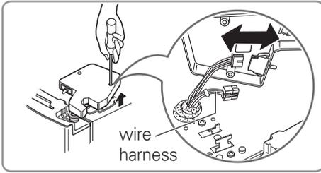
1. Open the door. Remove the top hinge cover screw.
