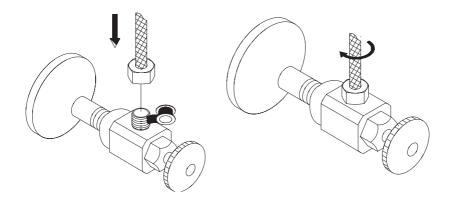
Connect and tighten waterlines (I) to angle stops. Turn on the angle stops and check for leaks (**DO NOT TURN FAUCET ON**)
