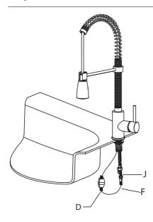
Connect spray hose (F) to supply hose (J) and tighten. Attach weight (D) to lowest point vertically on spray hose (F)
