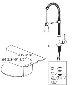
Remove mounting hardware assembly (C)
