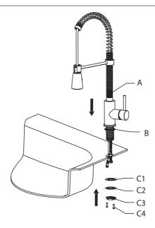
Insert faucet body (A) into hole on deck or sink with base (B) attached. Attach mounting hardware assembly (C)
