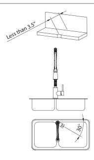
If the distance between the faucet hole and the wall is less than 3.5", position the faucet lever 30 degrees to 90 degrees off of the wall to allow for full operation
