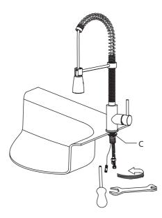
Adjust faucet body. Secure mounting hardware (C) with wrench and Phillips head screwdriver
