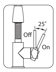
1. Pull the lever to the right to turn on the water. Push to the left to turn off
