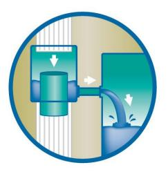
The Diverter channels rainwater from the downspout to the Rain Barrel reservoir
