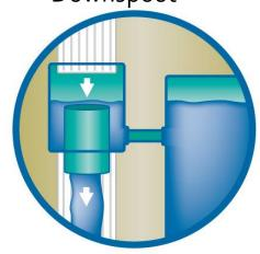
Downspout water diverter eliminates reservoir overflow. When rain barrel reservoir is full the rainwater flows down the downspout
