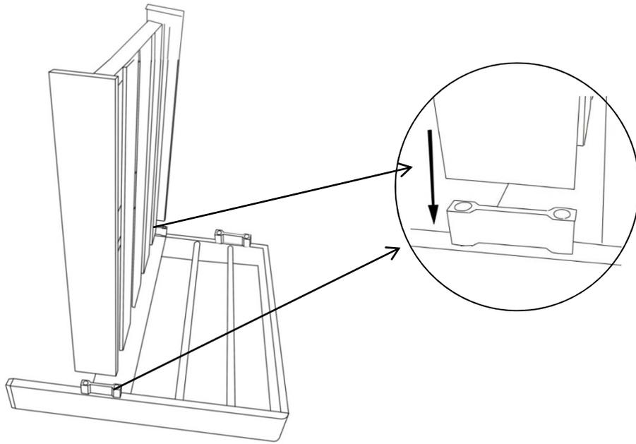
Insert the Seat(C) onto the Side Panel(A), as shown in the picture.
