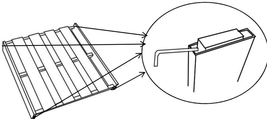
Take out the silders in the four ends of the Seatboard(C ) using Allen Key(E ).
