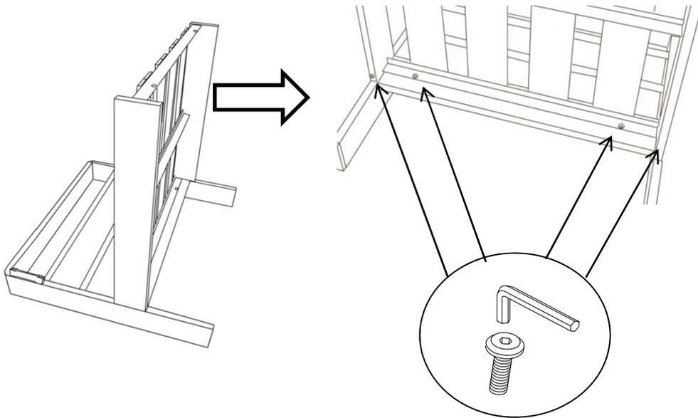
Attach Seat(C) and Side Panel(A) using Bolt(D) with Allen Key(E) as shown in the picture.
