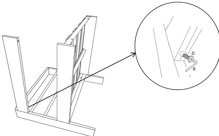
Attach Back Support Bar(B) to Side Panel(A) using Bolt(D) with Allen Key(E).
