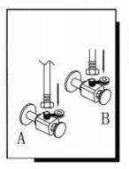
3.Attach two flexible hoses to water supply.
