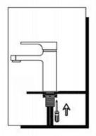
2. Tighten by screwing two screws if needed.
