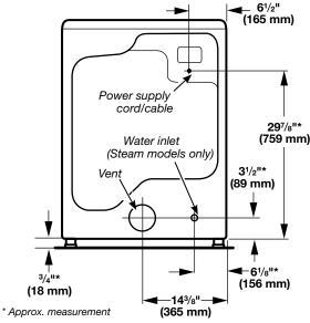
**NOTE:** Most installations require a minimum of 5" (127 mm) clearance behind dryer for exhaust vent with elbow. See "Venting Requirements."
