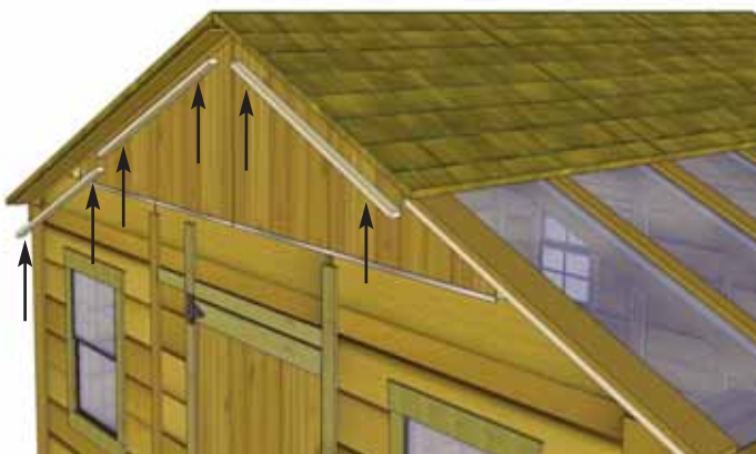
84. Attach Facia Cleat (3/4" x 1 1/2" x 36 1/2") centered on underside of Short Roof plywood, flush to edge. Attach Facia Cleats (3/4" x 1 1/2" x 40") to underside of Long Roof plywood, 1/2" from ends and flush to edge. Repeat this step on the rear side of shed.
