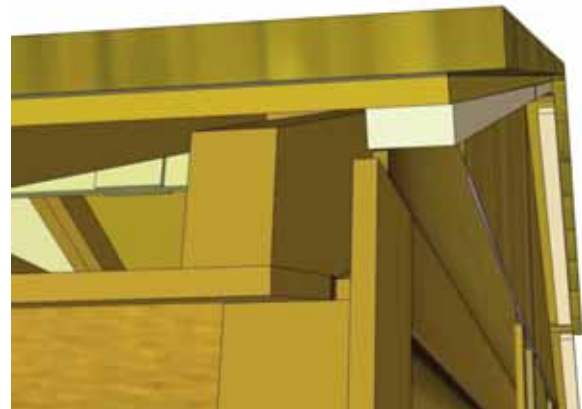
84. Attach Facia Cleat (3/4" x 1 1/2" x 36 1/2") centered on underside of Short Roof plywood, flush to edge. Attach Facia Cleats (3/4" x 1 1/2" x 40") to underside of Long Roof plywood, 1/2" from ends and flush to edge. Repeat this step on the rear side of shed.
