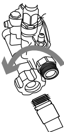
Figure 2-9. Connect Water Supply Hose
