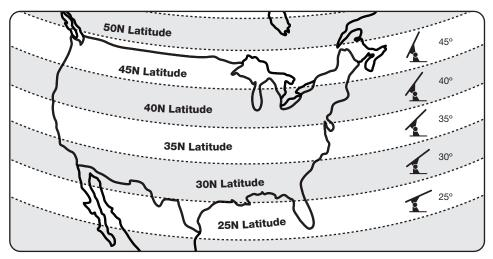
Orient the solar panel at approximately the same angle as the latitude of your location, taking into consideration the angle of the surface you are mounting it to.
