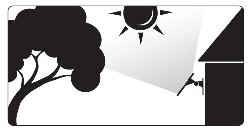
Mount the solar panel facing due south with direct line of sight to the sun. Be sure to avoid any potential obstructions, such as buildings or trees, that may cast a shadow on the panel during the day.
