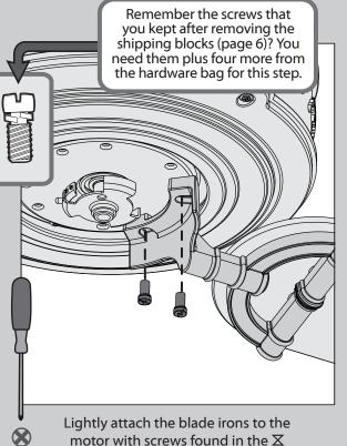
motor with screws found in the X hardware bag, then securely tighten after both screws are attached.
