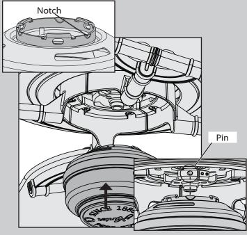
Raise the light kit to the bottom of the fan. Align the notch on the mounting ring on the top of the light kit with the pin in the mounting bracket on the bottom of the fan.
