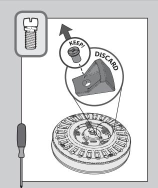
Remove the shipping blocks from the motor. Save the screws. They will be needed for blade iron installation.
