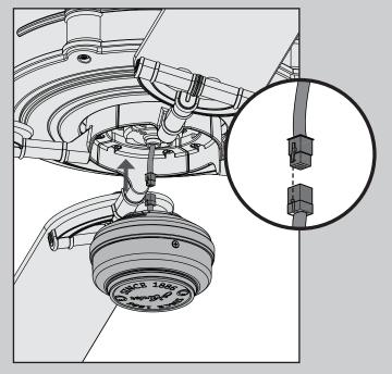
Connect the plugs from the fan and light fixture. Make sure to line up the colored markings on the connectors and that the connectors are latched together.
