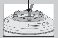
Push the **connector and excess wire** into the hole at the top of the light fixture.
