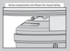
Give the fixture a gentle, counterclockwise turn to ensure the fixture is secure and that the locking pin has engaged.
