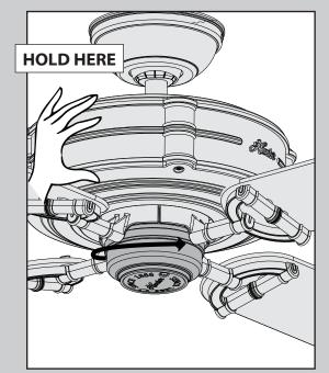
Hold the fan body stationary and rotate the light fixture clockwise to engage the locking pin.
