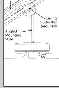
Use **Angled Mounting** to hang the fan from a vaulted or angled ceiling.
