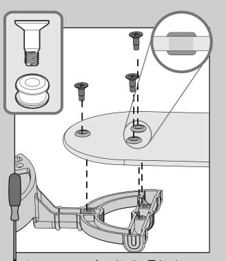
Insert grommets found in the ■ hardware bag into the holes in the blades, then secure each blade to a blade iron with screws found in the ▲ hardware bag.
