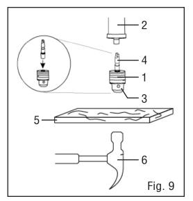
**CAUTION:** To avoid damaging the chuck, make sure the jaws are completely recessed into the chuck. Do not use a metal hammer to drive the chuck onto the arbor or into the spindle.
