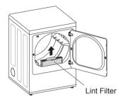
To clean, open the dryer door and pull the lint filter straight up. Then:
