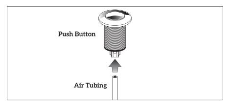
B. Measure the distance from the push button to the dedicated location where the Push Button Power Wall Adapter will be installed . If required, cut the air tubing and insert the open end to the female connector on top of the Push Button Power Wall Adapter.
