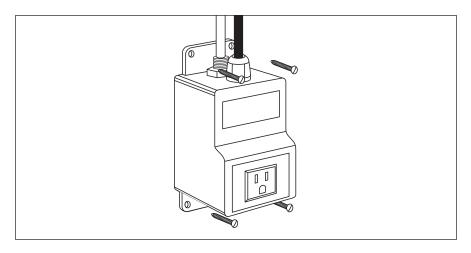
B. Plug the Push Button Power Wall Adapter's power cord into a grounded 120V AC outlet.
