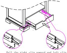
Pull the right clip upward and left clip downward at the same time, then draw the drawer box out.
