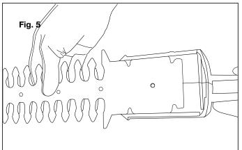
**NOTE:** You may need to manually move the blade or gear shaft in order to align the gear shaft with the gear in the center of the unit.
