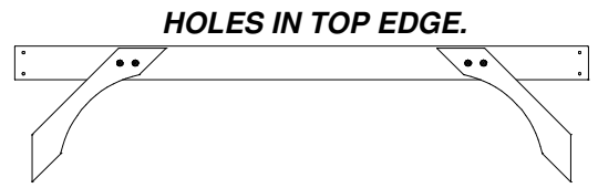
(2) 90" JOIST - SUPPORT ASSEMBLY
