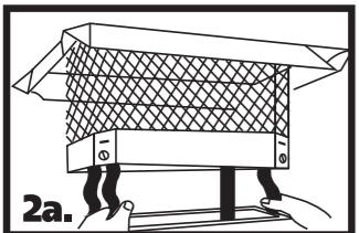
**STEP 1.** Insert one screw into the round hole located in each mitered corner of the chimney cover band. (Just start the screw into the hole a few turns until all 4 screws are started.)
