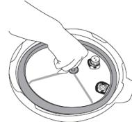
**Note:** If the gasket is not positioned properly, the unit will not build pressure. The silicon gasket must always be properly positioned. Check periodically to make sure that it is clean, flexible, and not cracked or torn.
