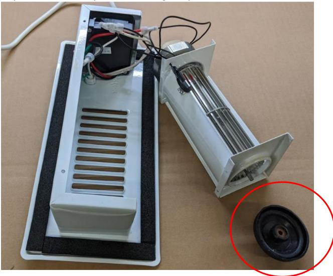
Step 3: Pull the fan away from the housing to expose the lubricant reservoir
