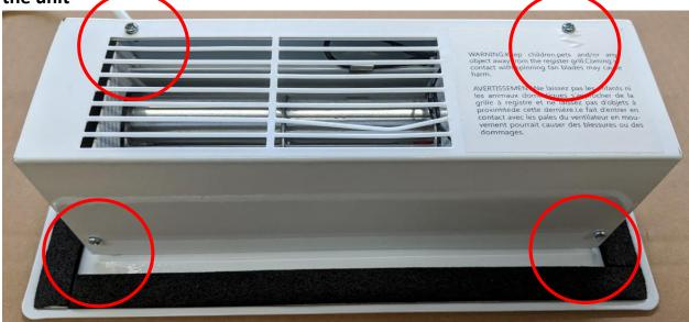
Step 2: Remove the product housing to expose the interior
