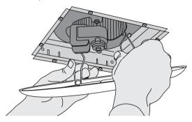
3.) Your existing fan may be attached in several ways. Look for attachment screws in the ceiling and remove. Your fan may also be attached on the attic side, which will require you to access it from the attic. Locate attic attachment screws and remove.
