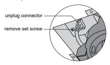
10.) Remove the electrical cover set screw and slide open the electrical enclosure. Connect wiring using the provided QUICK CONNECTS (U.S.A.) or WIRE NUTS (Canada).
