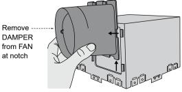
3.) Attach DAMPER to ducting. Tape DAMPER to ducting with duct tape. Set the connected DAMPER and ducting in the ceiling opening, then set the FAN in the ceiling opening as well.
