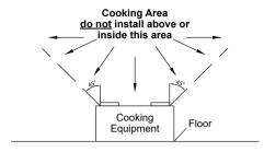
Do not install ventilation fan in areas where the duct work will require configuration as shown.
