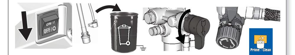
With the trigger lock in locked position, unthread spray tip and (2) guard assembly from gun. Place in waste pail for further cleaning.
