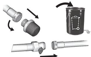
**TO SAVE PAINT IN HOSE**: Trigger gun into paint pail, 5 turn Prime/Spray Valve forward to **SPRAY** and turn Power Switch **ON**. When water comes out of gun, keep gun triggered and aim into waste pail. Continue to flush until water runs clear.
