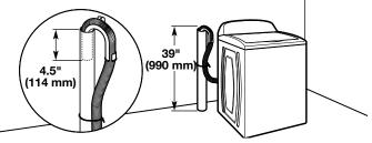
Minimum diameter for a standpipe drain: 2" (51 mm). Minimum carry-away capacity: 17 gal. (64 L) per minute. Top of standpipe must be at least 39" (990 mm) high; install no higher than 96" (2.44 m) from bottom of washer. If you must install higher than 96" (2.44 m), you will need a sump pump system.
