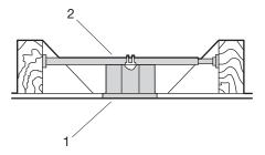
To hang your fan where there is an existing fixture but no ceiling joist, you may need an installation hanger bar (2) (not included) as shown above.
