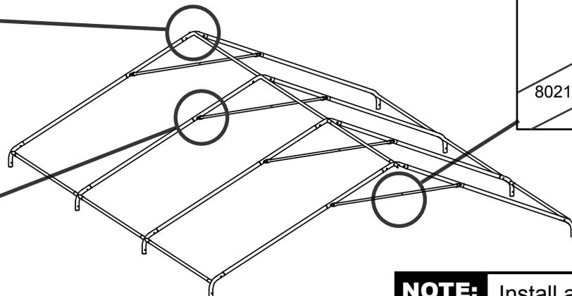
**NOTE:** Install all carriage bolts with the nut toward the center of the frame.
