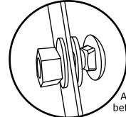
Assemble fasteners to bracket before hanging on keyhole slots.
