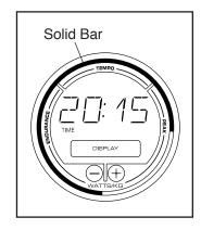
**To set a power output target**, press the Watts/ Kg increase and decrease buttons until the desired power output target appears in the display.
