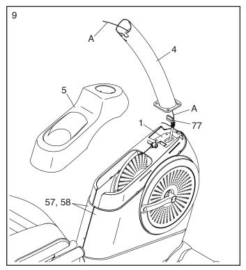
10. **Tip: Avoid pinching the Main Wire (77).** Hold the Upright (4) against the Frame (1). Attach the Upright with four M8 x 15mm Screws (24). **Start all the Screws, and then tighten them.**
