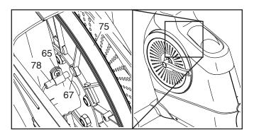
Next, rotate the Pulley (75) until a Magnet (67) is aligned with the Reed Switch (78). Slide the Reed Switch slightly toward or away from the Magnet. Then, retighten the M4 x 12mm Washer Head Screw (65).
