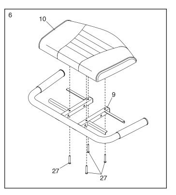
Attach the Seat Frame (9) to the Seat Carriage
