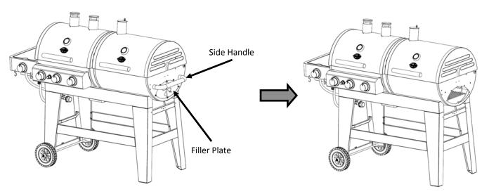
**Step 2:** Attach SFB to Charcoal Grill Body using (6) 1/4-20 x 1/2" Hex Bolts, (2) 1/4-20 x 2 1/4" Hex Bolts, (8) 1/4-20 Hex Nuts, and (2) Spacer Tubes. The Hex Bolts go from inside the SFB and Hex Nuts on inside of Charcoal grill Body.
