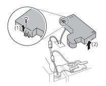
2 Detach the wire harness (1). Unscrew the ground wire (3) on the InstaView model only.
