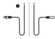
Connect the MC4 ends of the halved cable **4** to the compatible MC4 ends of the solar panel **G** cables. (Mark the end of the positive panel cable with a piece of tape to help distinguish polarity during connection.)
