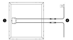
Connect the bare wire end of the positive cable 4 to the "SOLAR +" input of the charge controller 1. Connect the negative bare end to the "SOLAR -" input. Now, you can mount the PWM-165 to an indoor wall or within a NEMA-3R rated enclosure.
