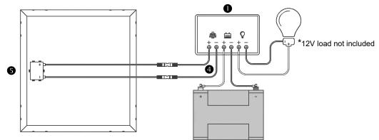
Remove the panel covering. In good sunlight, the charge controller's **0** "BAT %" should increase to 100%. Once the battery is fully charged and the controller is set to "LOAD ON," the system will provide power through the load control output or through the two USB ports. If an inverter is added to the system, it must be connected to the battery bank, and not to the charge controller.
