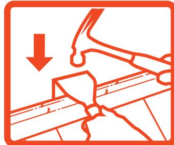
Position Trim Puller's front face against the wall with the sharp edge on the seam where trim meets the wall. For best results start at the end of baseboard strip.
