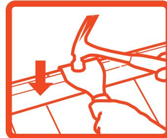
Strike top of Trim Puller with hammer or hard mallet driving the Trim Puller between the trim and the wall. The wedge will begin to separate the trim from the wall.
