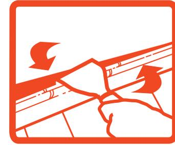
Once the Trim Puller is wedged between the trim and the wall gently pry the trim away from the wall creating a gap of approximately 4" to 8". Repeat Steps 2 – 4 moving the Trim Puller along the wall in 12" increments or as needed. The gap in Step 4 will increase with each pull until removed.
