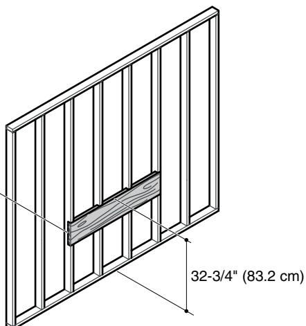
**NOTICE:** To properly secure the vanity, the top of the required 2x6 backing material must be 32-3/4" (83.2 cm) from the finished floor.
