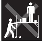
REMOVE OR FASTEN TOOLS, MATERIAL OR EQUIPMENT BEFORE MOVING. NEVER MOVE A SCAFFOLD WITH WORKER WITHIN.
