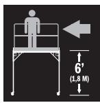
GUARDRAILS RAILS MUST BE INSTALLED ON ALL OPEN SIDES OF A WORK PLATFORM WHERE A PERSON COULD FALL FROM A HEIGHT OF 6 FT (1.8 M) OR MORE
