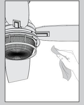
When cleaning the fan, use soft brushes or cloths to prevent scratching. Cleaning products may damage the finishes.
