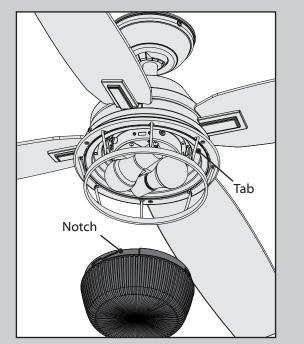
Lift the globe and align the notches in the globe with the tabs in the light kit. Attach the glass bowl to the light kit by twisting it clockwise until it snaps into place.
