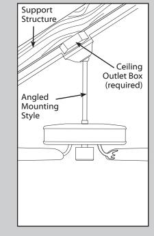
Use **Angled Mounting** to hang the fan from a vaulted or angled ceiling.
