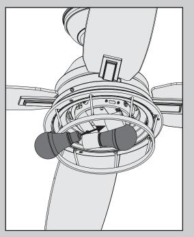
Install a bulb into each of the sockets. When necessary, replace with bulbs of the same type and wattage.
