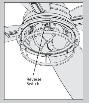
**To switch the direction of air flow,** move the reverse switch to the opposite position. You will need to remove the light cage and glass to do so.
