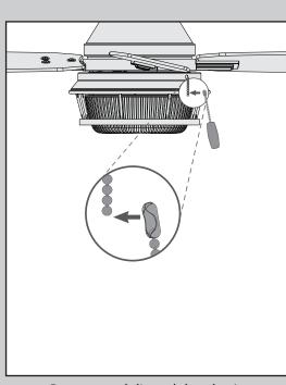
Remove and discard the plastic connectors from the ends of the short pull chains Connect the appropriate pull chain pendant to each of the short chains coming from the light kit. The fan pull chain controls the speed: from high to off. The light pull chain controls the light fixture: on and off.
