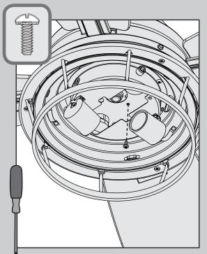
Insert a third light kit assembly screw, found in the ≡ hardware bag, into place and tighten all three screws securely.
