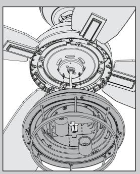
Align the keyhole slots in the top of the light kit assembly with the partially installed assembly screws. Wrap the keyhole slots around the screws and twist counterclockwise.
