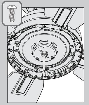
Partially install two light kit assembly screws, found in the ≡ hardware bag, halfway into the motor housing as shown. It does not matter which two screw holes you choose.
