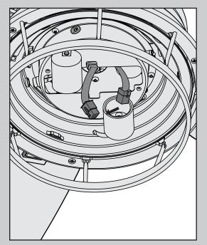
Feed the 9-pin plug connector coming from the bottom of the motor housing through the center hole in the light kit assembly. Connect it to the plug connector found in the switch housing area of the light kit assembly. Make sure to line up the colored markings on the connectors.
