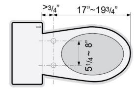
Note: the Swash Ecoseat 100 is designed to fit elongated toilets only, however this model will in fact fit select round fixtures. Please reference the fit diagram for size verification. The Swash Ecoseat 100 will not fit French curve fixtures.
