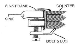
NOTE: When frame is used with Stainless Steel or Porcelained Steel sinks, use a pad between bolt end and sinks. This will provide assurance against damage to sink deck. Pads 3/4" x 3/4" may be made of plastic, laminate surfacing or metal (not provided).
