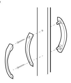
these steps for the bottom of the handle then fully tighten the 2 screws. Snap the cover back onto the female handle.
