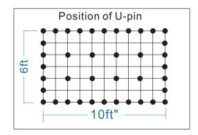
Black dots are the positions of U-Pins. 1 U-Pin for every 1ft for Out layer. 1 U-Pin for every 2ft for inner layer.
