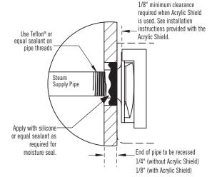
CAUTION Consult with supplier of acrylic, fiberglass and other non-heat resistant enclosures for recommended steamhead location. Use Acrylic Shield PN 103938 / 103938SQ. See instructions provided with steam shield. (An acrylic shield is not available for the iSteam steamhead.)
