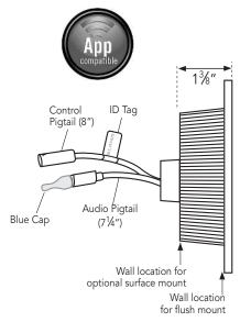
iSteam controls flush mount in the steam/shower enclosure through a 5-1/4" wide x 3-9/16" high hole. iSteam controls can also be surface mounted. They are suitable for use with an available iGenie® control. Available in black or white.
