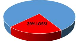
Source: http://www.energycodes.gov/rescheck UA Calculations applied to a 1000 sq/ft. attic with a pulldown ladder installed
