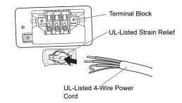
5 Transfer the dryer's ground wire from behind the green ground screw to the center screw of the terminal block.
