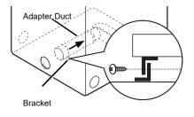
3 Insert the 4-inch (10.2 cm) elbow through the rear opening and press it onto the adapter duct. Be sure that the male end of the elbow faces down through the hole in the bottom of the dryer. Secure it in place with duct tape. Attach the cover plate to the back of the dryer with the included screw.
