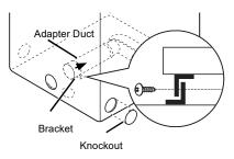
3 Preassemble a 4-inch (10.2 cm) elbow to the next 4-inch (10.2 cm) duct section, and secure all joints with duct tape. Be sure that the male end of the elbow faces AWAY from the dryer. Insert the elbow/duct assembly through the side opening and press it onto the adapter duct. Secure it in place with duct tape. Be sure that the male end of the duct protrudes 1.5 inches (3.8 cm) to connect the remaining ductwork. Attach the cover plate to the back of the dryer with the included screw.
