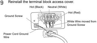
Reinstall the terminal block access cover.
