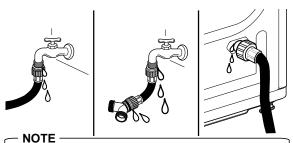
• If any leaks are found, shut off the water faucet, remove the hose and check the condition of the rubber seal.
