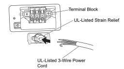
5 Attach the two hot leads (black and red) of the power cord to the outer terminal block screws.
