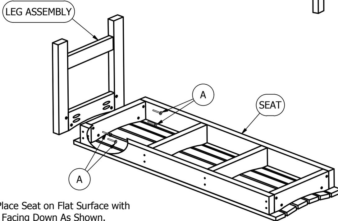
**1)** Place Seat on Flat Surface with Top Facing Down As Shown.
